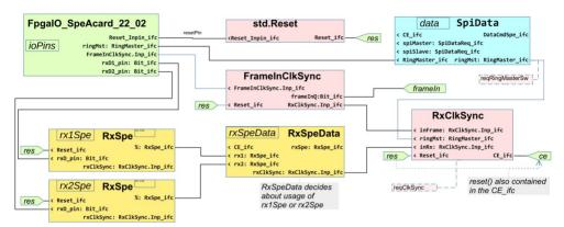
Figure 3: Example for a Module Diagram
