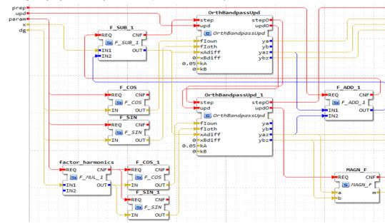
Figure 12. OrthBandpass in a filter application
