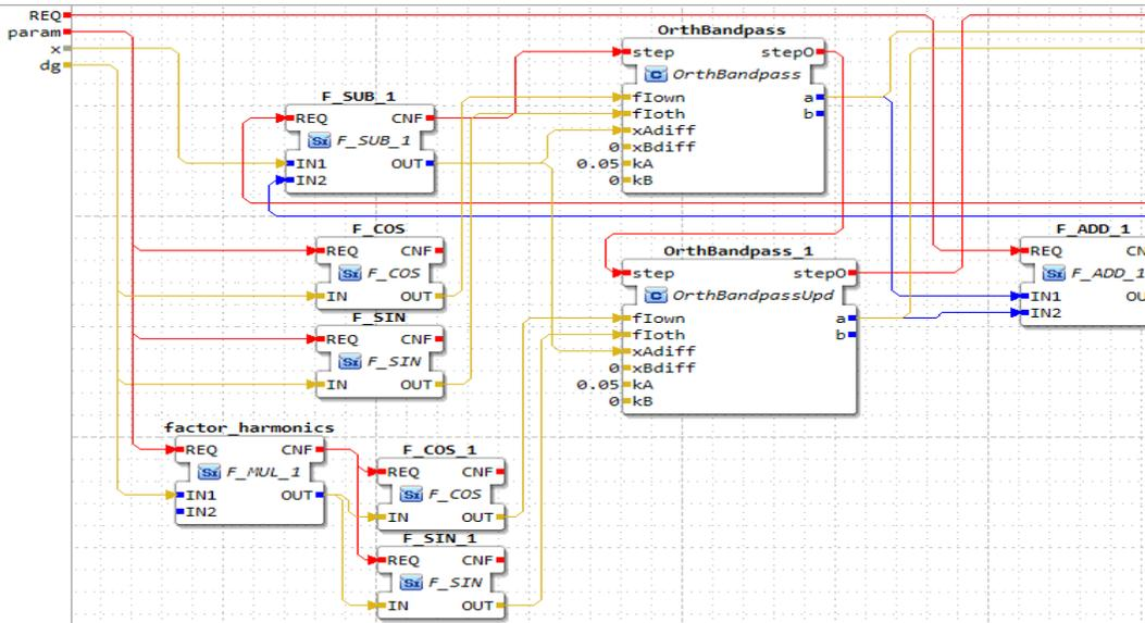
Figure 11. OrthBandpass in a filter application
