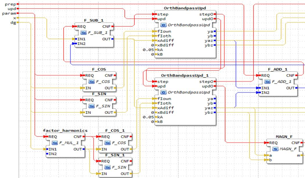
Figure 12. OrthBandpass in a filter application
